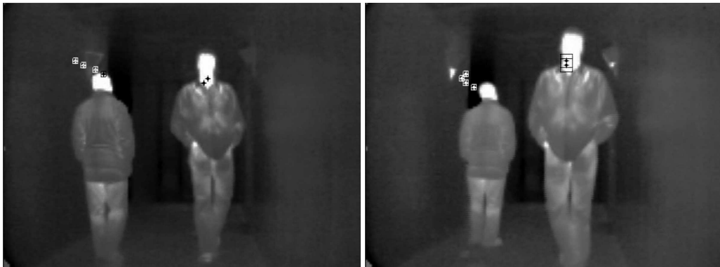
Figure 2. Two images of thermally distinctive objects being tracked by the PQS. The left image shows a person in a hallway walking with a bottle of hot water. The bottle is tracked below, while the face of the person is tracked separately. The person is walking backward. The right image shows a person holding a cup of coffee. Notice how the fingers obscure and segment the cup into three parts that are all tracked separately.
